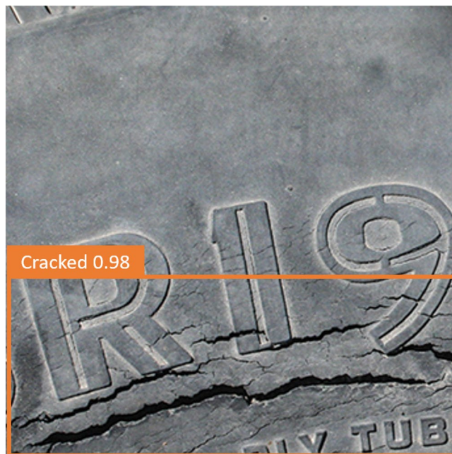
Figure 15. In YOLOv7, the detection results of large cracks in defective tires are 98%.
