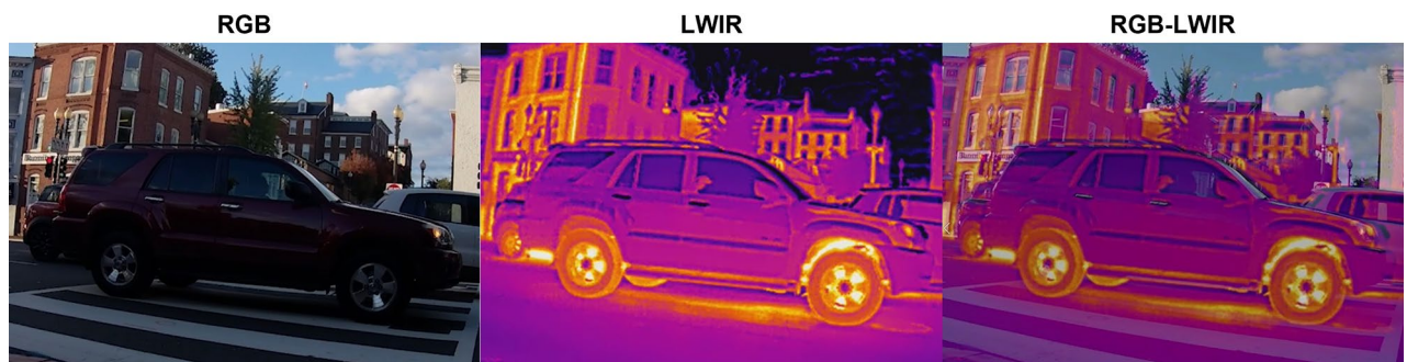
Figure 5. An example of an RGB image (left), an LWIR image (middle) and a RGB-LWIR fused image (right).
