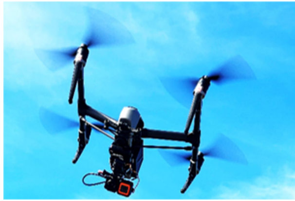
Figure 4. The primary air-based platform used for this research (the DJI Inspire 2) carrying the RGB-LWIR payload.
