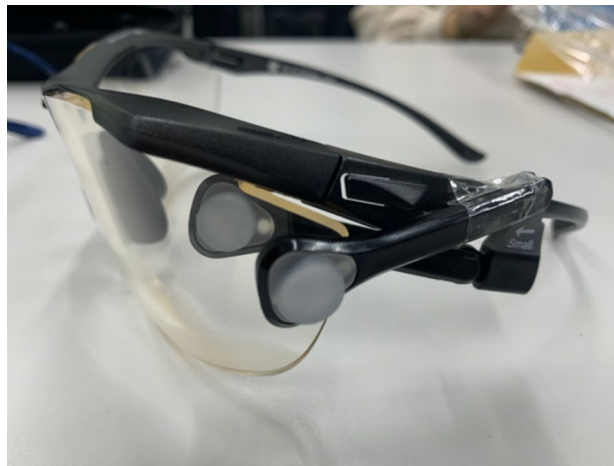
Figure 1. Eye dosimeter (DOSIRIS™) attached to the left side of the lead glass (inside and outside of the lead glass).
