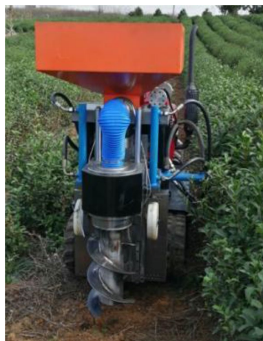
Figure 8. Field test of the single-spiral ditching and fertilizing machine.
