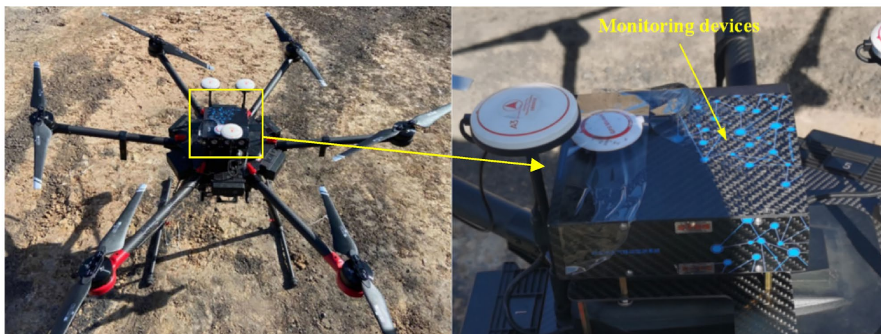
Figure 3. DJI M600pro with monitoring equipment.
