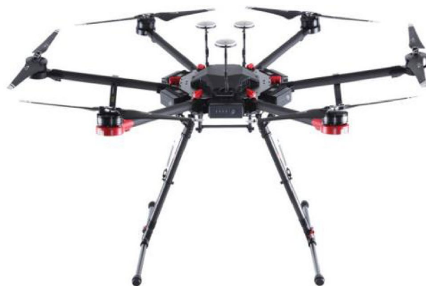
Figure 2. DJI M600pro UAV.
