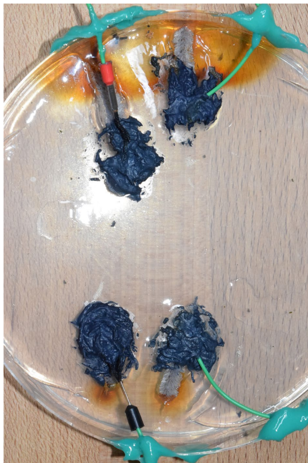
Figure 5. PEDOT Polymer electrode on agarose plate. Right: green metal leads directly in the electrode, Left: conductive textile interface between electrode and metal wire. Electrode diameter: 2 cm.
