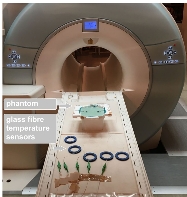
Figure 3. Setup with MRI. In the foreground, the temperature sensors are attached to the table, behind them is the head phantom with the electrodes and cables.
