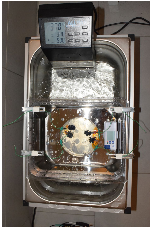
Figure 4. The climate chamber setup. The outer water basin is held on a constant temperature. The inner basin is filled with water underneath a perforated metal-plate. A petri dish with the PEDOT polymer electrodes is placed above the metal plate. A short piece of pipe cleaner was inserted inside the agarose for better adhesion of the electrode (the pipe cleaner's inner wire leads to orange corrosion spots on the agarose). Recording wire endings are outside the chamber (green leads). The data logger is in direct vicinity to the petri dish.
