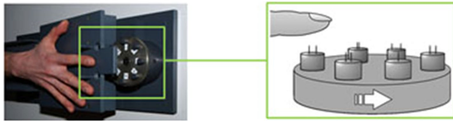
Figure 1. The two-point discrimination device used in the study. Seven different inter-pin distances (0.7–2.5 mm) and 1 control pin (0 mm) are presented to the index finger in random order.
