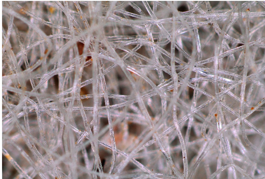
Figure 2. Microscopic image of nonwoven surface of virgin GCL at 32× magnification.
