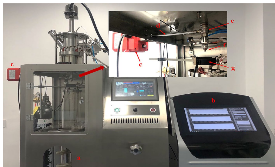
Figure 2. The setup used in the dripping experiments. (a) dripping machine, (b) self-designed software carrying out the data processing and controlling, (c) electric actuator, (d) valve rod, (e) drop valve, (f) drop head, and (g) laser micrometer.
