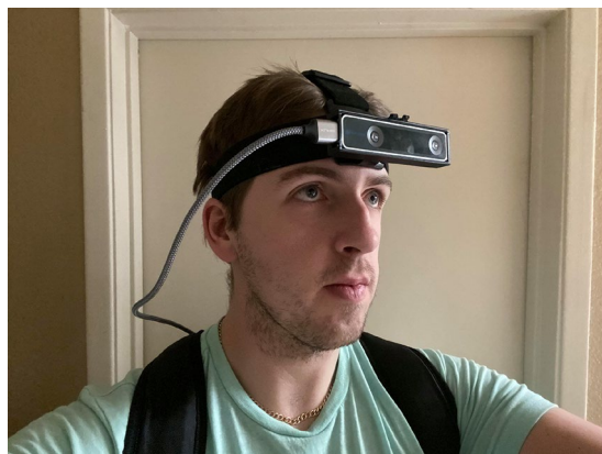
Figure 1. Recording equipment. The T265 measures 6 degree of freedom (6DOF) position of the camera relative to the world, and is worn on the head by a participant over 5 h. The camera plugs into a lightweight laptop worn in a backpack.
