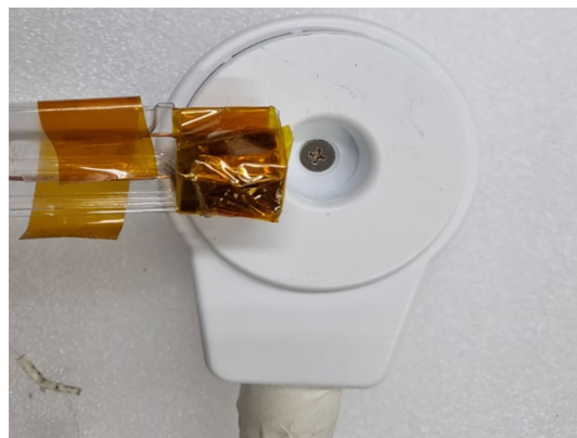
Figure 13. Measurement setup of electric field intensity of fabricated coil.
