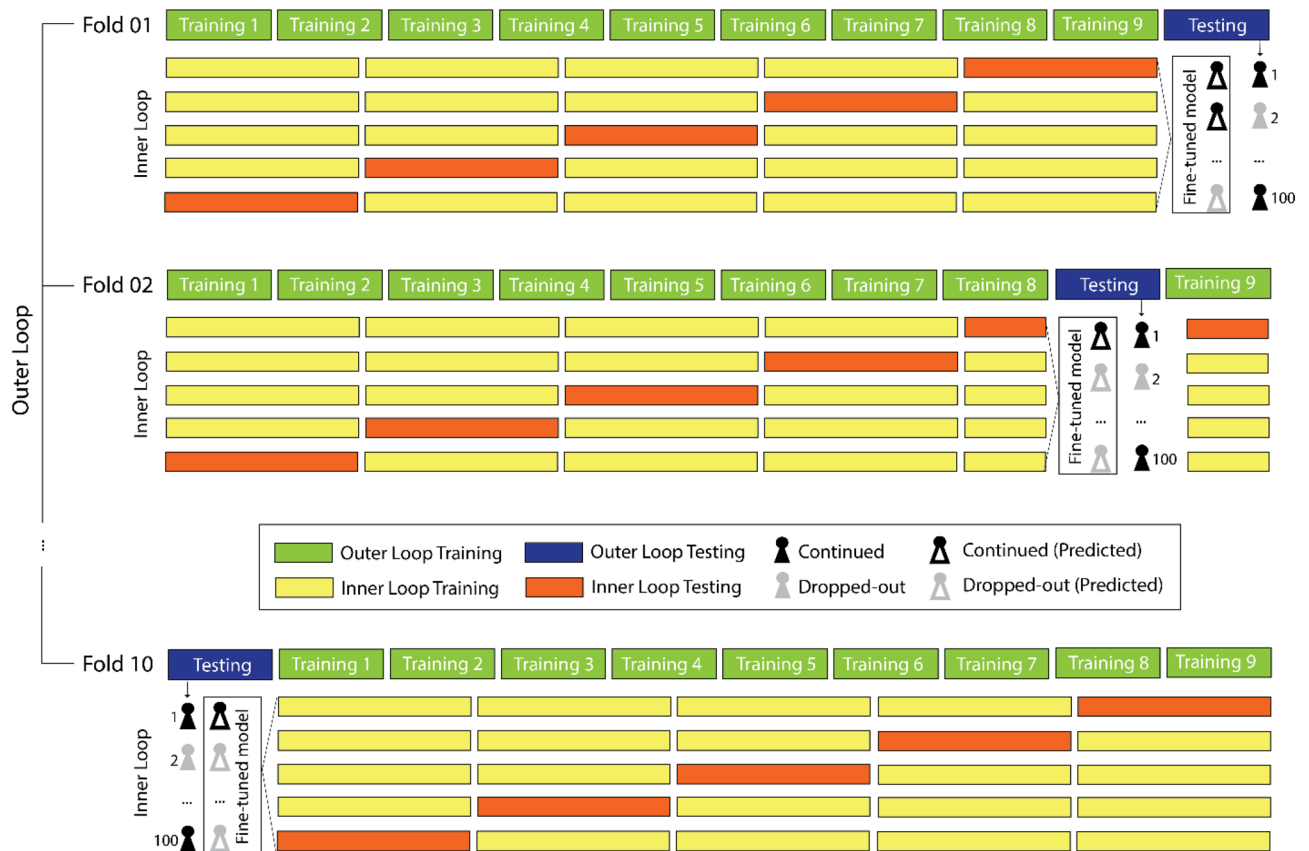
Figure 1. Schematic cross-validation procedure for out-of-sample predictions. The figure shows a tenfold cross-validation in the outer loop which is used to estimate the overall performance of the model by comparing the predicted outcomes for each student in the previously unseen test set with their actual outcomes. Within each of the 10 outer loops, a fivefold cross-validation in the inner loop is used to finetune model hyperparameters by evaluating different model settings.
