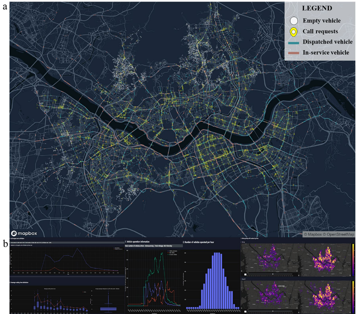
Figure 2. Final implementation of DTUMOS in Seoul Metropolitan Area. (a) a simulation visualization using deck.gl framework (b) a system performance report containing level of service (LOS) of the system, vehicle operation information, and spatial analysis. See a simulation visualization and a system performance report in a web browser. The map is created using Mapbox GL JS v.2.12.0 ( https://www.mapbox.com/ ).
