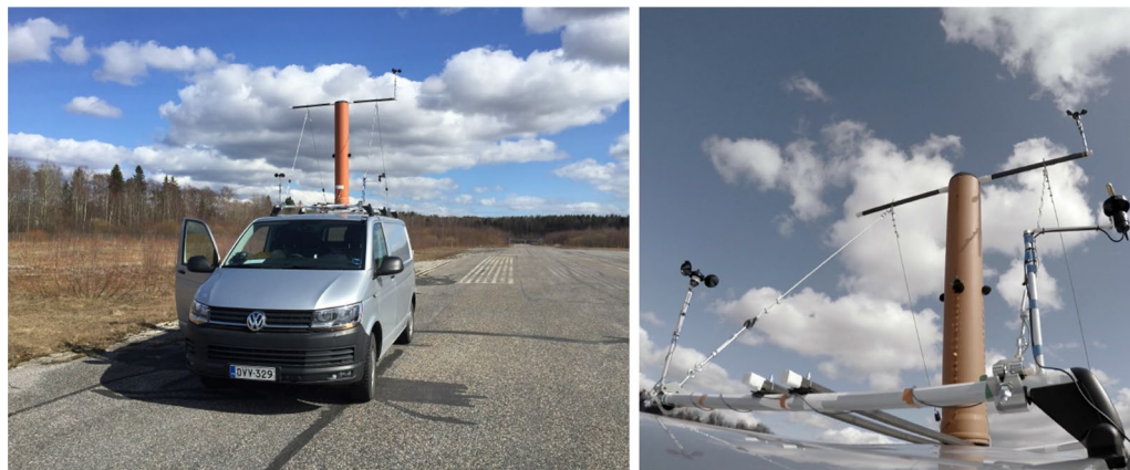
Figure 4. Still images of the measurement rig on the roof of the van and GoPro footage of 0^\circ (upwind) measurement setup.
