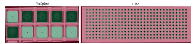
**Figure 11.** Grid Detection. The automated grid estimation using Grid Screener is shown for wellplate and DMA input images. The grid elements are marked via crosses (centroid) and green overlays. A red overlay denotes the background.
