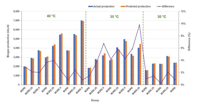
**Figure 3.** Comparison of predicted biogas production and average of actual data. M2: OLR of swine manure = 2 g-VS/L/day; R0.25: VS ratio of swine manure/waste kitchen oil = 0.25.
