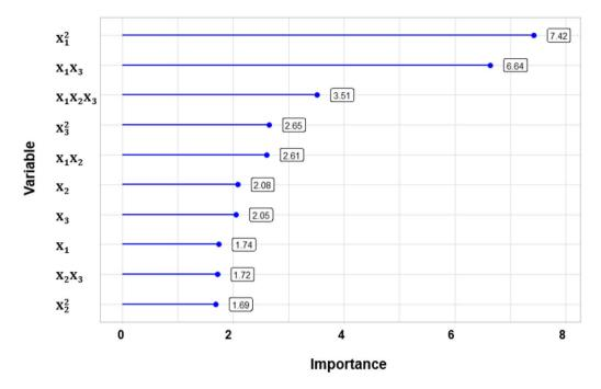
Figure 2. The importance score of each variable in the quadratic model.  $X_1, X_2, X_3$  represented VS loading rate of swine manure, waste kitchen oil/manure ratio and temperature, respectively.
