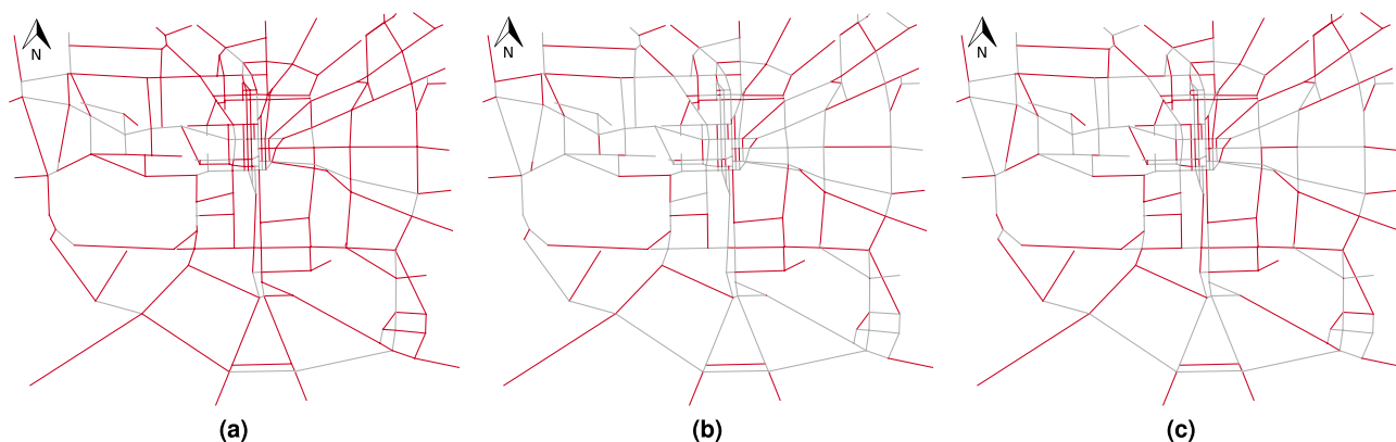
Figure 12. Final QGIS map output of roads that need to be monitored (red segments) by placing a traffic sensor based on: (a) scenario 1 with optimal weights, (b) scenario 2 with optimal weights, and (c) scenario 3 with optimal weights.
