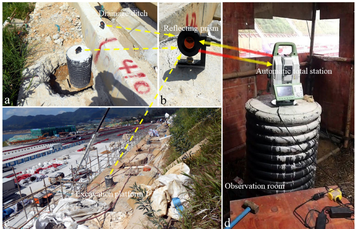
Figure 8. Automatic total station deformation monitoring system. (a–c) Show the prisms placed in the field; (d) shows the automatic total station placed in the observation room.
