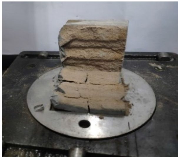
Figure 17. Significant compression failure of the shear failure plane.
