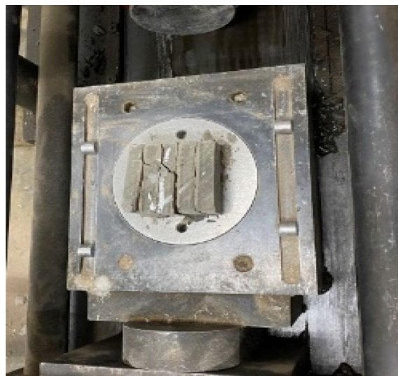
Figure 16. Breakage of the cemented rock column along the joint surface.
