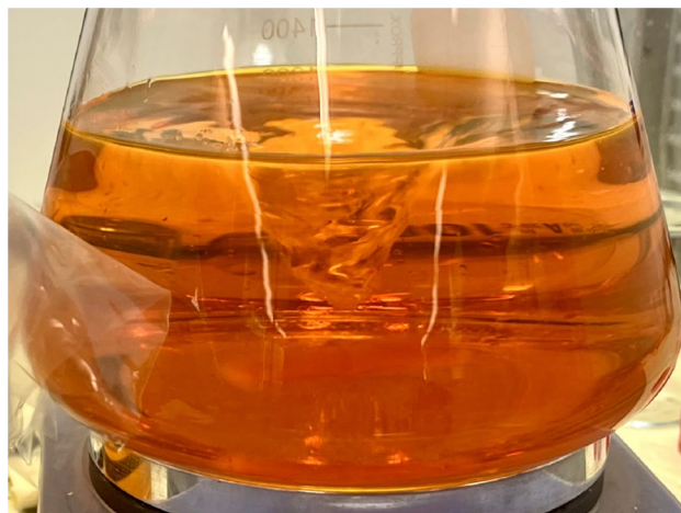
Figure 2. Sample Sipdril 4/0 stained with Nile red on a magnetic hot plate stirrer.
