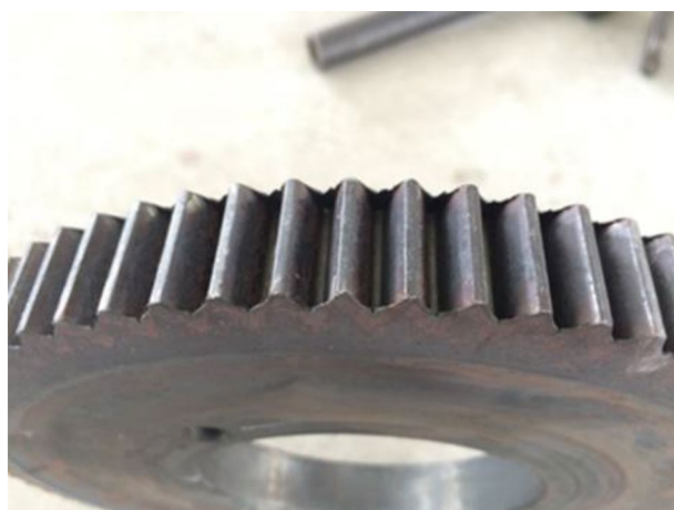
Figure 14. The formed tooth of the workpiece without metal folding defect using finishing roller device.
