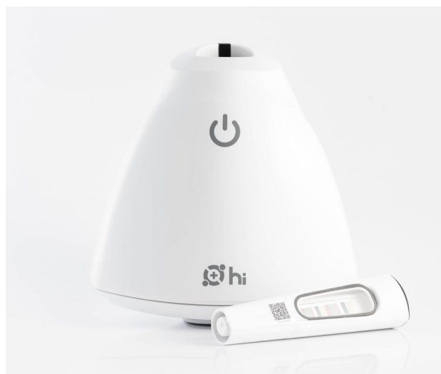
Figure 1. Hilab Flow, a device capable of performing lateral flow and vertical flow point of care tests.
