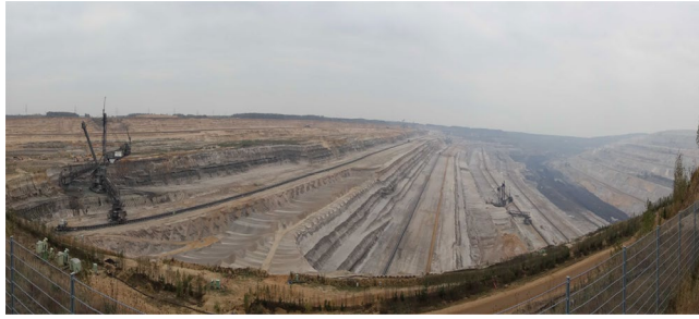
Figure 1. View of the extraction side of the lignite opencast mine Hambach (left hand side) with a surface of 85 km 2 and depth 400 m created with coal excavator and dumping site (right hand side) 1 .
