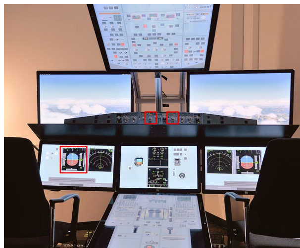
Figure 3. The iSim A321 cockpit. Primary flight display (left) and hardware panel with heading dial (centre left) and vertical speed dial (centre right) for required inputs are marked in red.
