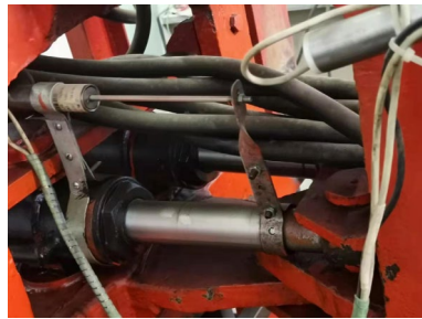
Figure 2. Swing DOF in the construction robot.
