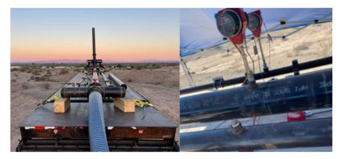
**Figure 5.** Metering and release trailer (left) has four pipes (0.5-in., 2-in., 4-in., and 8-in.), each leading to a distinct metering location allowing a different dynamic range of release volumes. The three larger pipes used a QuadraTherm 640i insertion meter (right), with upstream 8.5 m straight run of pipe to ensure sufficient flow stabilization for all pipes. The 0.5-in. pipe was not used in this study.
