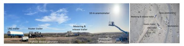
**Figure 4.** The experimental setup in panorama (left). Liquefied natural gas was reheated before flowing through a metering and release trailer. An aerial photograph of the site (right) [courtesy of Bridger Photonics Inc.]. Note that the release trailer is ~45 m from liquefied natural gas (LNG) trailer and ~45 m from workstation and anemometer. Adapted with permission from<sup>36</sup>.
