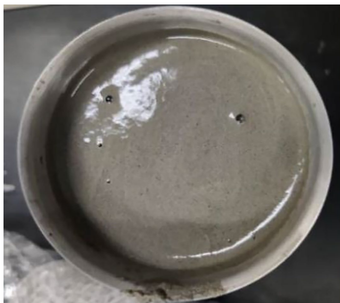
Figure 5. Appearance of cement slurry with the combination of chemical-induced nitrogen-foam additive and glass beads.
