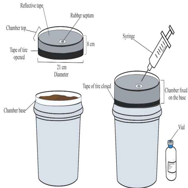
Figure 6. Static chamber details and instruments for GHG collection in the dung beetle trial.
