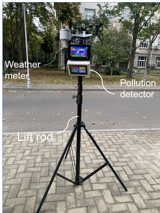
Figure 2. The analytical diagram of self-developed multifunctional lifting environmental detector.
