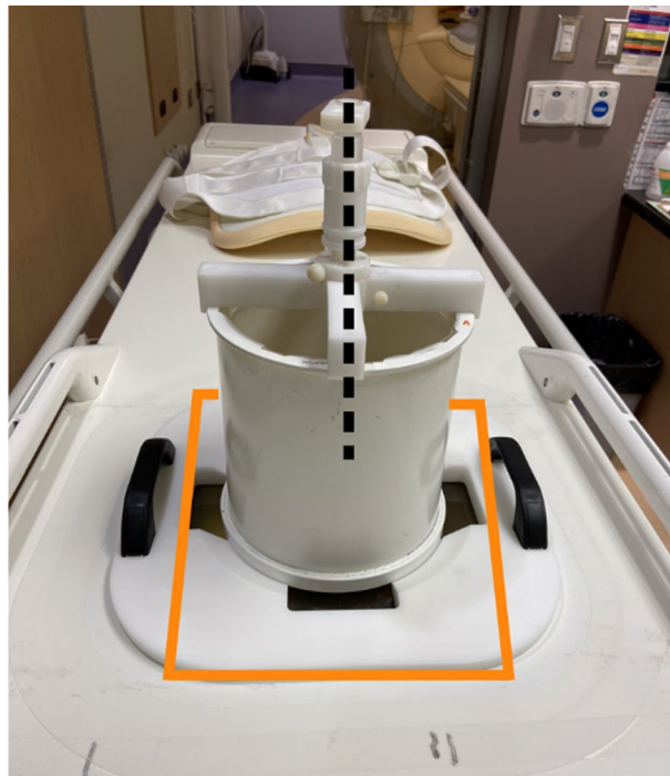
Figure 1. A custom build plastic housing was installed on a hollowed Sonalleve quality control phantom. The dotted black line indicates where a needle hydrophone and wiring could be threaded into degassed water 6 cm above the window membrane (highlighted in yellow).
