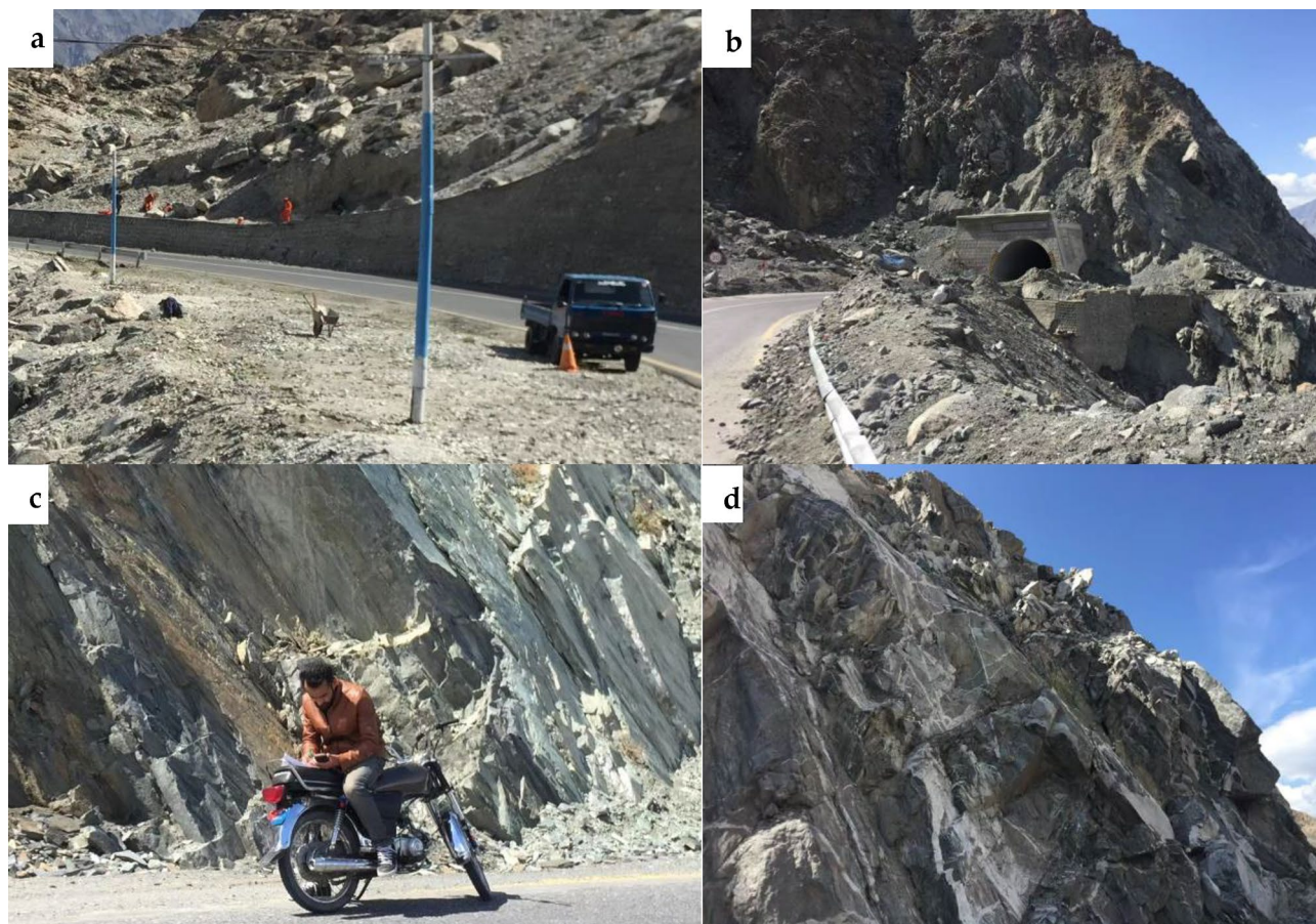
Figure 14. Investigation of various types of landslide during a field visit. (a) The Frontier Works Organization (FWO) clears the road after a rock fall in the Nagar District. (b) Debris flow in District Gilgit. (c) Using GPS to obtain actual landslide's location. (d) Rockfall in District Hunza.
