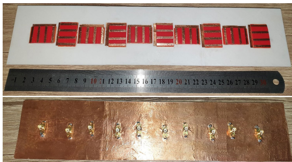
Figure 9. Front and back views of the fabricated two cloaked interleaved arrays.
