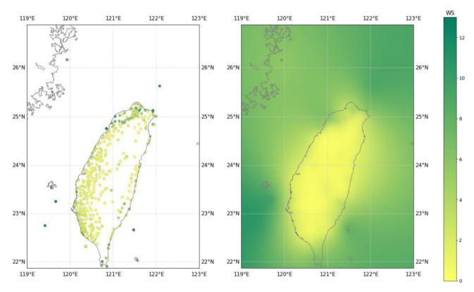
**Figure 1.** Left side: CWB and buoy monitoring stations. Right side: distribution of ocean wind dataset after kriging interpolation.
