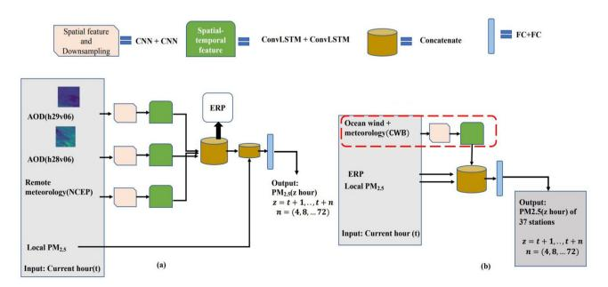
**Figure 2.** STRI model components STRI\_fe (a) and STRI\_p (b) with modifications indicated by red dashed line.
