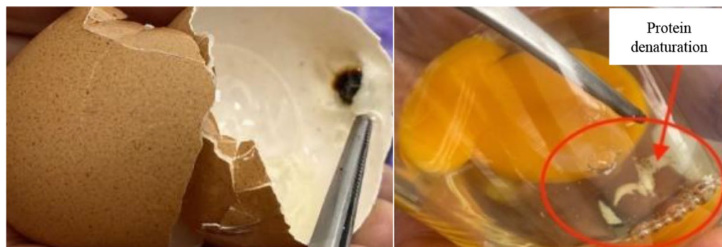
Figure 1. Burn mark on eggshell and protein denaturation in egg white.
