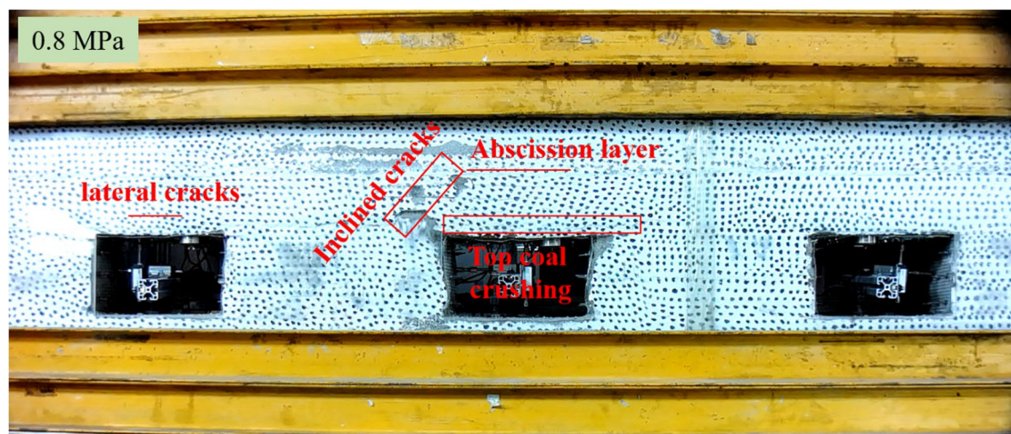
Figure 18. Failure characteristics of surrounding rock of each roadway at a loading pressure of 0.8 MPa.
