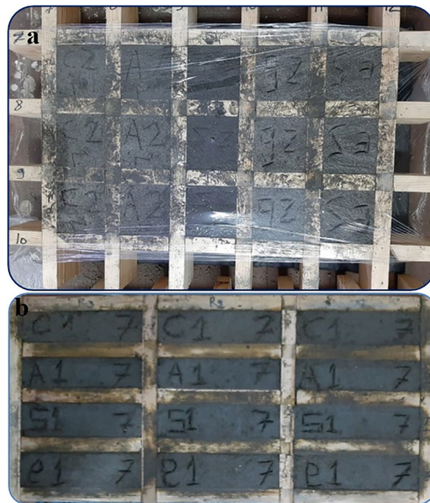
Figure 10. Cube wood molds containing the mortar (a), Prisms (b); Cement: sand = 1:3, Ash/Cement = 0.1, Bacterial culture/cement = 0.5.
