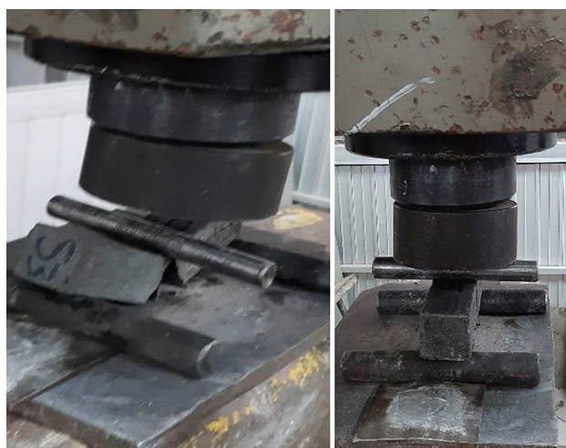
Figure 13. The used electrohydraulic bending and compression testing machine.
