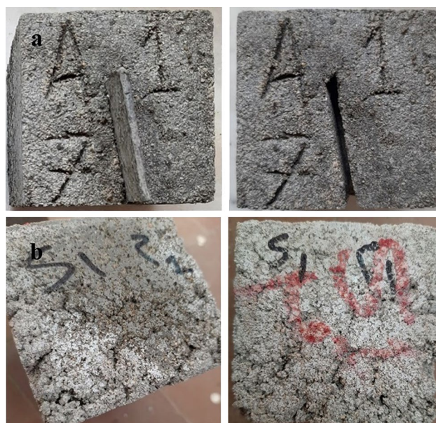
Figure 12. Cracks by a plate of steel (a), Natural cracks (b).
