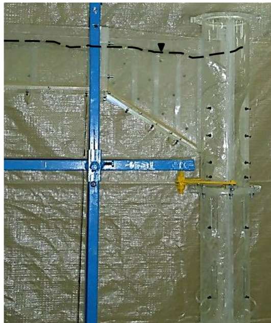
Figure 5. Observed disturbance in the formation of vortex flow for Q > 33 l/s.
