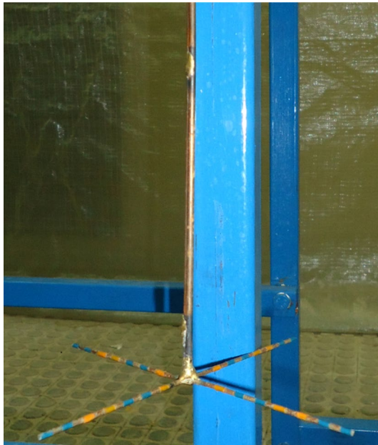
Figure 3. A device manufactured to measure the thickness of the vortex flow.
