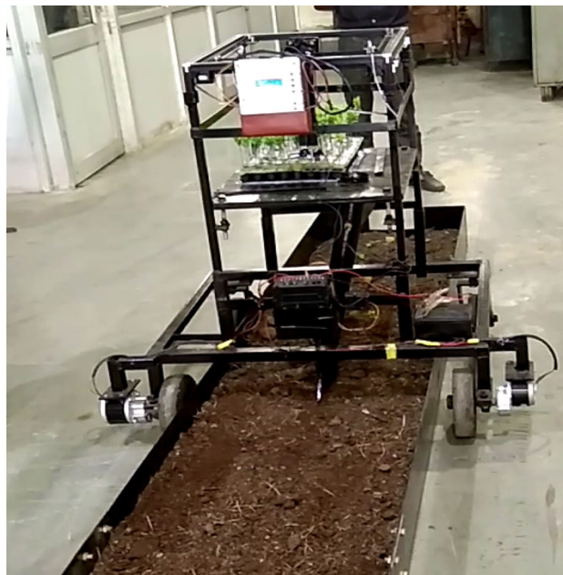
Figure 9. Test setup of robotic transplanting with plug seedlings.
