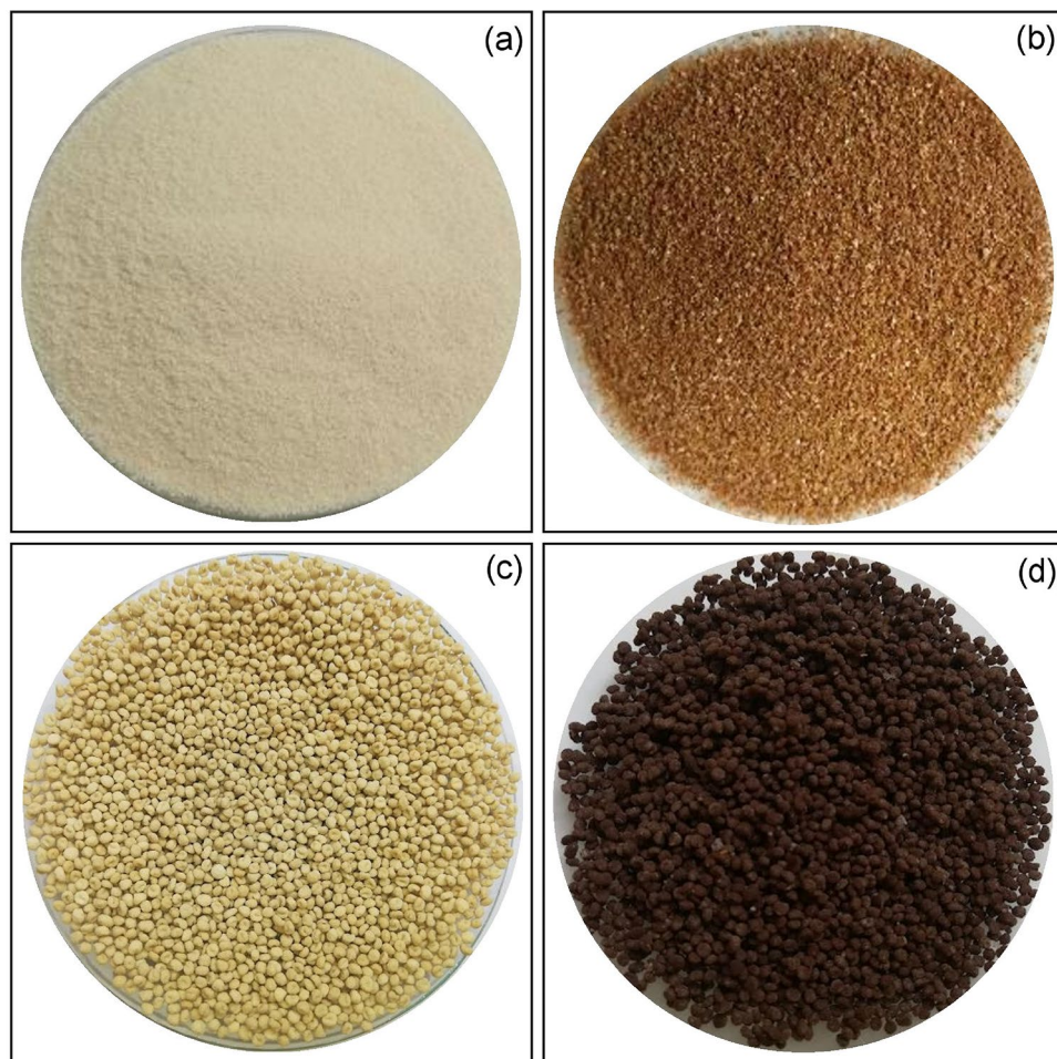
Figure 1. The physical characteristics of (a) sugarcane bagasse powder (SB), (b) sugarcane bagasse powder doped iron(III) oxide-hydroxide (SBF), (c) sugarcane bagasse powder beads (SBB), and (d) sugarcane bagasse powder doped iron(III) oxide-hydroxide beads (SBFB).
