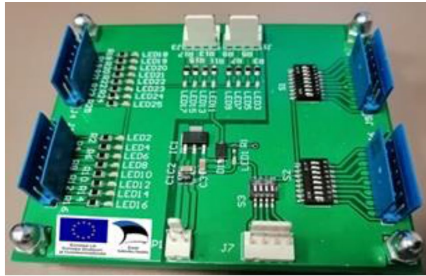
Figure 6. Logic test bench board.
