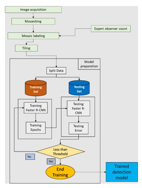
**Figure 2.** Flowchart of the steps followed to train and test the Faster R-CNN model from the expert observer counts. Results of the trained detection model were then used for comparisons with the experienced observer counts.
