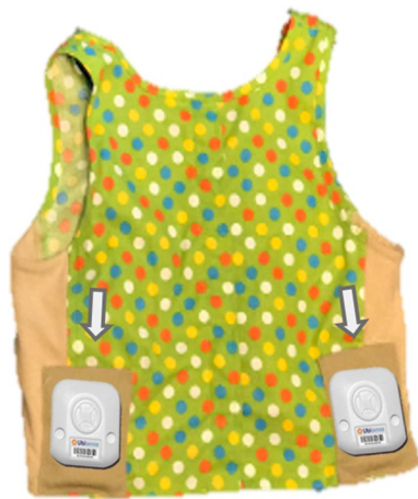
Figure 6. Vest and RFID trackers. Vest with pockets for Ubisense tags (1" × 1" × 0.36").
