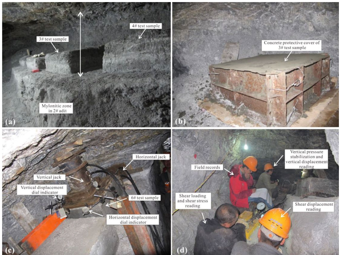
Figure 5. Process of in-situ shear test (a) Field pictures of 3# and 4# test samples, and mylonitic zone in adit; (b) Concrete protective cover of 3# test sample; (c) Device of in-situ shear test and 6# test sample; (d) Field record of in-situ shear test.
