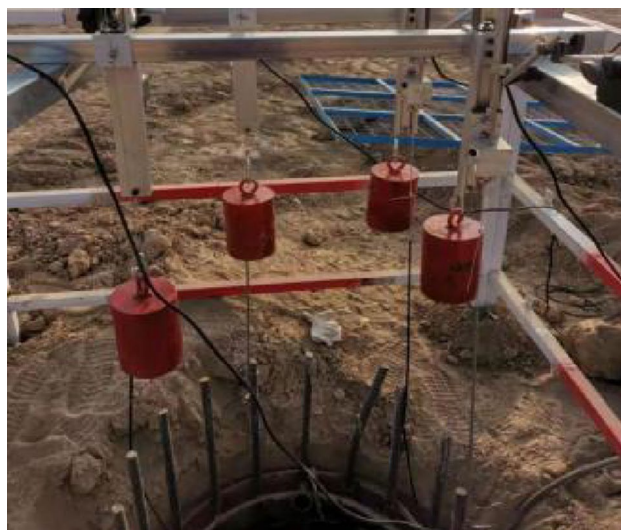
Figure 4. Displacement measuring device.
