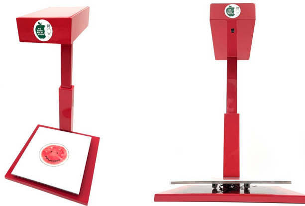
Figure 10. A prototype of an integrated plate waste tracker. It consists of load cells at the bottom to measure the weight of plate waste, and a camera at the top to capture an image of the plate waste before disposal, both of which are controlled by a ‘Raspberry Pi’ running a Python program.
