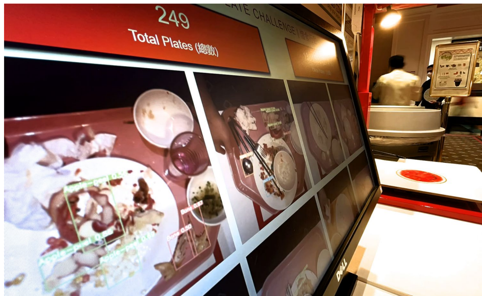
Figure 13. Clean plate challenge real-time display. It shows a live count of the total number of plates, the number of clean plates (with percentage to target) and the images of trays with bounding boxes drawn.
