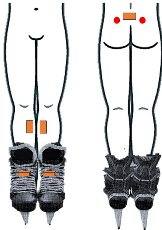
Figure 1. Five IMUs (orange boxes) were placed on the participants' pelvis, shanks and skates. Also, two pressure insoles placed in the skates and two retro-reflective markers on the PSISs (red circles) were used as a reference system for temporal event detection and stride length estimation, respectively.
