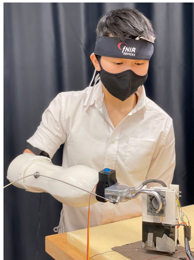
Figure 1. User grasps the brittle instrumented object with a myoelectric prosthesis featuring haptic shared control. An fNIRS headset over the forehead gathers neurophysiological measures of cognitive load.
