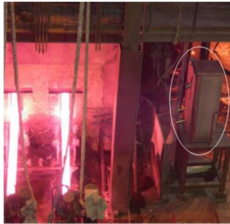
Figure 5. Temperature measurement verification of billet surface at secondary cooling outlet.
