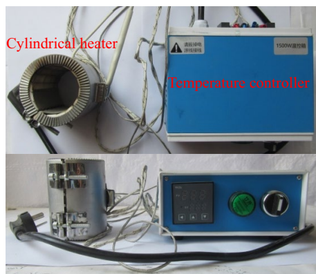
Figure 1. Segmented heating device for coal sample.
