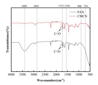
Figure 7. FTIR spectra of PAN and CMKN.
