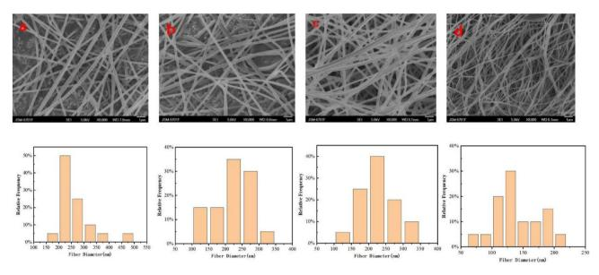
**Figure 3.** SEM images of electrospun CMKN fibers at different voltages and fiber diameters ((**a**):15 kV; (**b**):18 kV; (**c**):21 kV; (**d**):25 kV).
