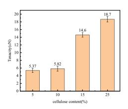
Figure 8. Tensile strength of a spinning fluid with different cellulose content.
