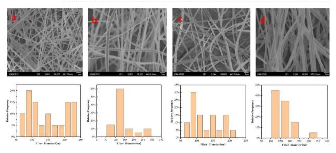
**Figure 5.** SEM images of electrospun CMKN fibers at different collection distances and fiber diameter distribution ((**a**):10 cm; (**b**):15 cm; (**c**):20 cm; (**d**):25 cm).
