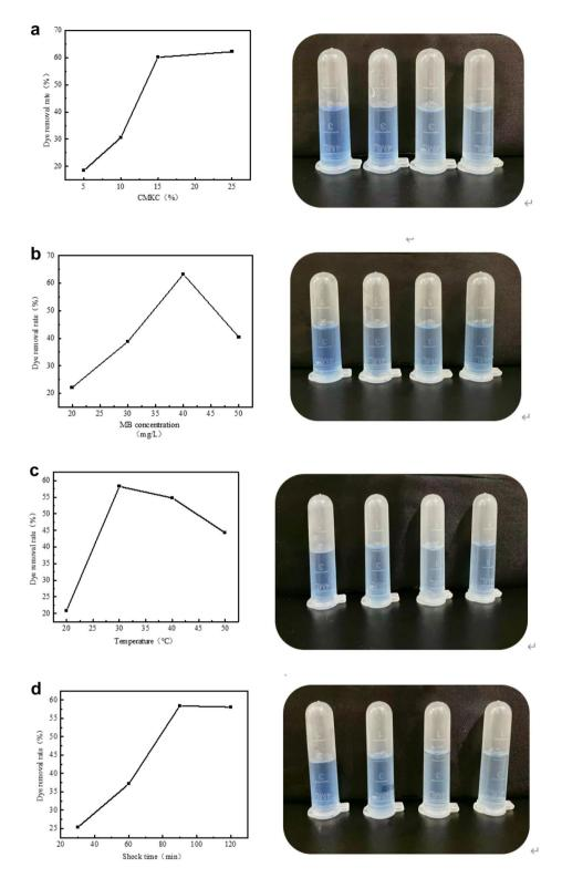
**Figure 9.** Effect of different factors on dye removal rate ((**a**): CMKC ratio; (**b**): MB concentration; (**c**): Temperature; (**d**): shock time).
