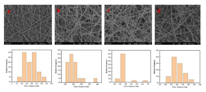
**Figure 4.** SEM images of electrospinning CMKN fibers at different pushing speed and fiber diameter distribution ((**a**):0.2 ml/h; (**b**):0.5 ml/h; (**c**):0.8 ml/h; (**d**):1 ml/h).
