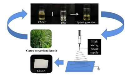
Figure 1. Route of electrospinning experiment.
